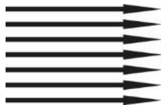
Alternate Line Direction: not marked Tool only travels in one direction
